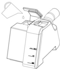
Figure 3-3 Filling water tank
